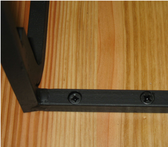
Close-up of the cage mounted to the base with 1 3/4 # 10 wood screws.
